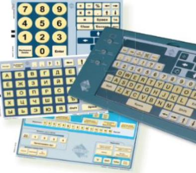
A collection of IntelliKeys assistive input devices. It includes a standard keyboard layout, a numeric keypad, and several specialized touch-sensitive pads with various key mappings and icons. One device has a large numeric keypad at the top. |
